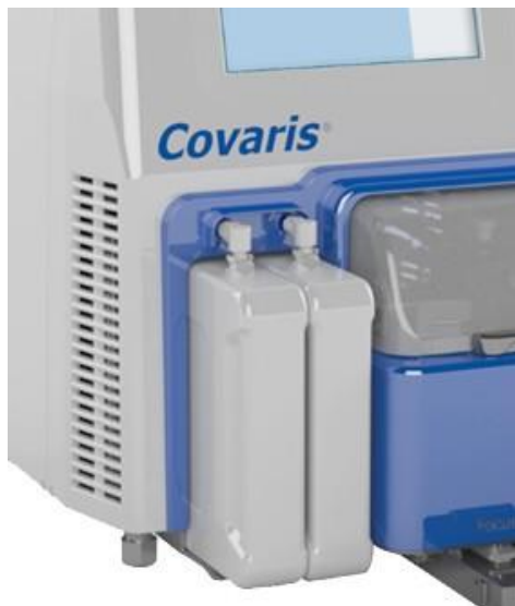
Figure 2.7 Bottles into Water Control Bay
