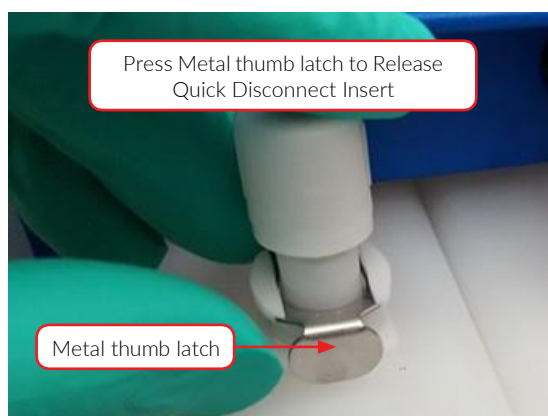
Figure 3.7 Releasing the Quick Disconnect Fittings
