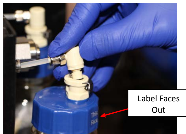
Figure 6 – Connecting the Bottle to the Water Works System
