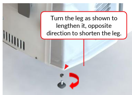
Figure 2.10 ME220 Leg Height Adjustment
