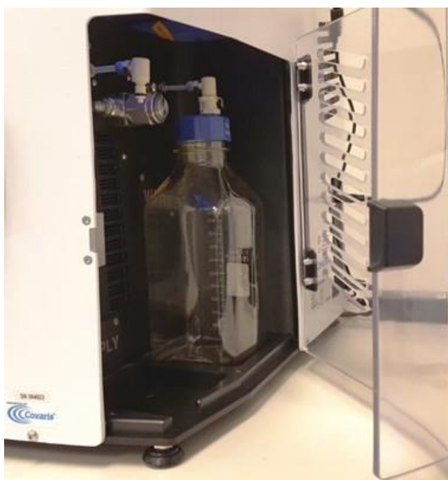
Figure 2.3 Placing Bottles into Water Works Bay
