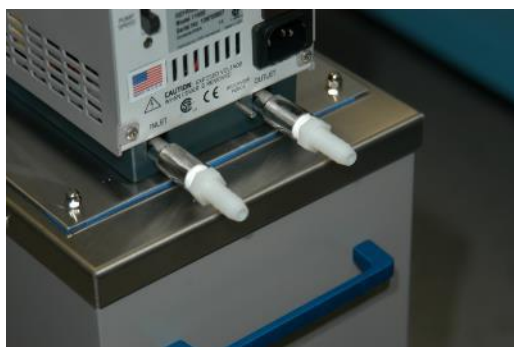
Barbed fittings installed on a chiller
