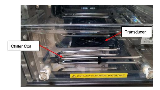
The **CH03 and CH04 chillers** pump fluid through hoses connected to the left side of the unit (see Setup) and then through stainless steel coils immersed in the water bath. These coils are visible as part of the Acoustic Assembly, surrounding the ultrasonic transducer.
