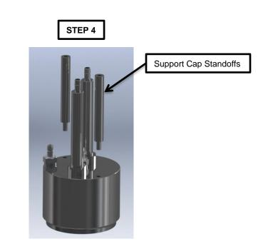
Position small orange O-ring inside groove of Feed through tube. Tighten tubes securely in place. Thread in Support Cap Standoffs in place, finger tight only.
