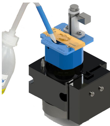
Figure 3.5 Easy filling with AFA-grade water
