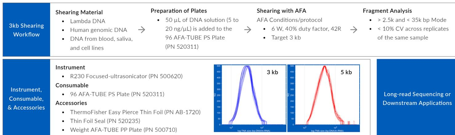
**Figure 1.** Overview of 3 kb DNA shearing workflow on the R230 Focused-ultrasonicator. A generalized workflow depicting the sequential steps involved in shearing process (top) and the required consumables and accessories (bottom) are designed for batch processing and are engineered for use with AFA Technology.
