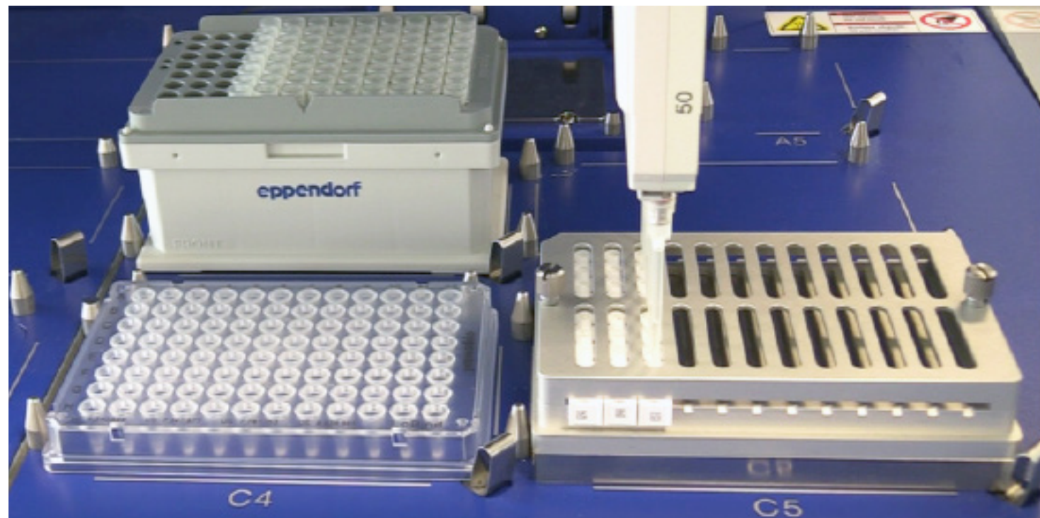
FIGURE 1: epMotion deck layout with Covaris 8 microTUBE-50 strips in the rack and adapter at position C5.
