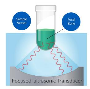
Figure 1: Isothermal processing through acoustic field control.
