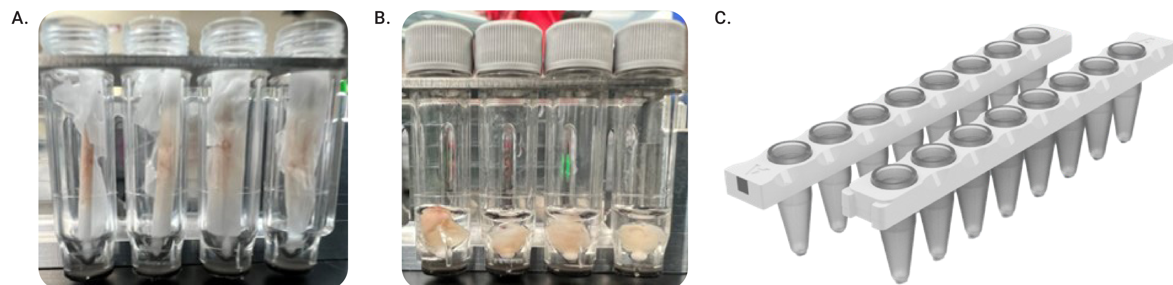
Figure 2: prepTUBE TPX and AFA-TUBE TPX. Several prepTUBE TPX loaded with a 10 µm FFPE kidney scroll and a single AFA Bead (A), FFPE kidney tissues after deparaffinization (B), and AFA-TUBE TPX Strips (C). Paraffin is removed from FFPE samples with a non-toxic Deparaffinization Solution. Following decrosslinking and tissue homogenization, the resulting lysate is transferred into the AFA-TUBE TPX for the remainder of the workflow.
