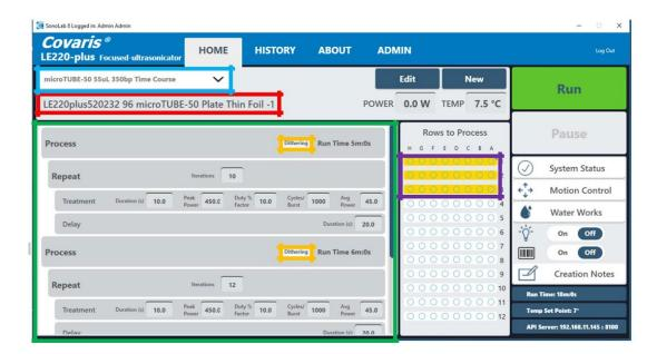
*Home Screen* for Time Course method. "microTUBE-50 55µL 350bp Time Course" uses the "LE220plus\_520232 96 microTUBE-50 Plate Thin Foil – 12mm offset" plate definition. The method includes repeat loops for 100 seconds, 120 seconds, and 140 seconds AFA treatment with 10 seconds pulses and 20 seconds delay for Rows 1, 2, and 3 respectively. Dithering is also included for this AFA treatment step.
